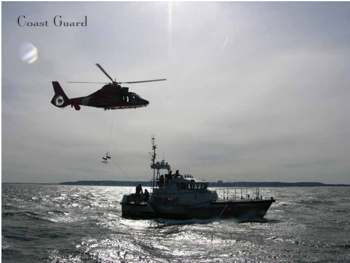
A Coast Guard Station Sandy Hook 47-foot Motor Lifeboat (which is able to completely roll upside down in heavy surf) practices basket hoists with a Coast Guard Station Atlantic City Dolphin helicopter. Pete Milnes Photo - PeteMilnes.com
